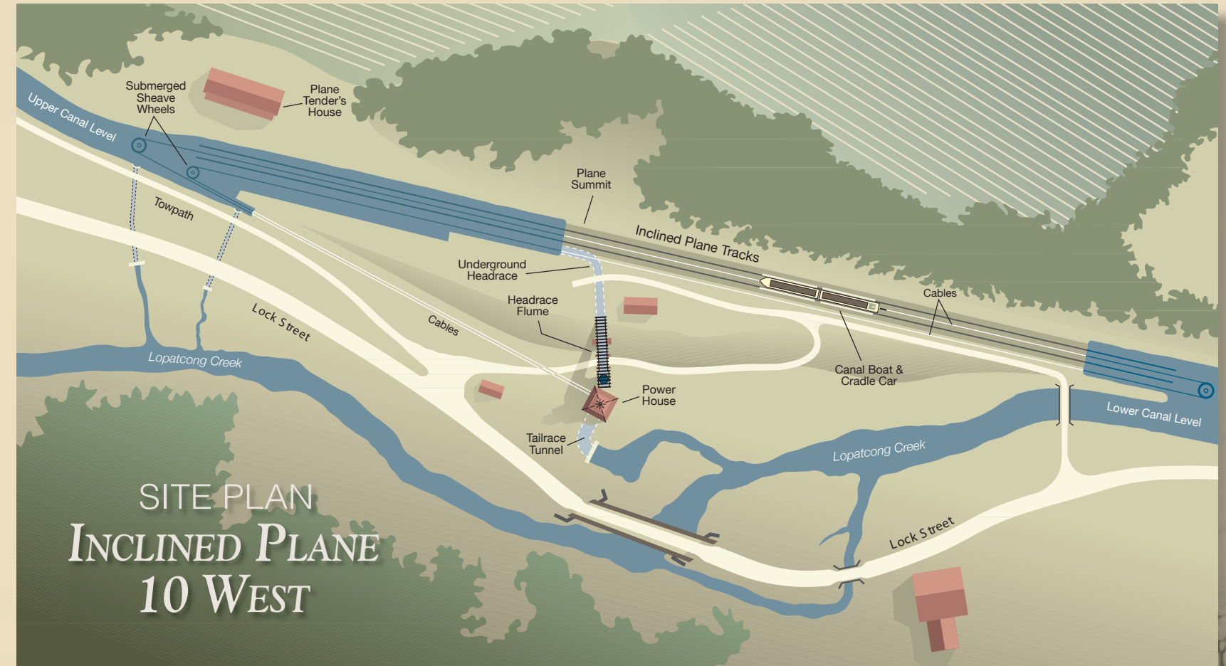
This site plan shows a detailed layout of the plane site. The upper canal level is on the left and the lower level on the right. In the center, a cradle car and canal boat are shown ascending the plane.
