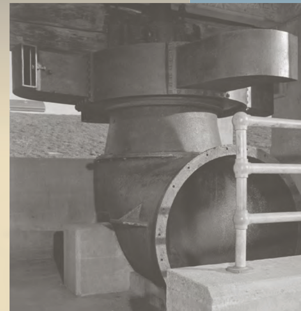
Several of the Morris Canal's Reaction Turbines survive today. The one pictured above came from Plane 3 East in Ledgewood and is now on display in Hopatcong State Park. Notice the curved nozzles that caused the rotor on top of the turbine to turn.
